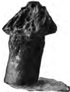
FIG. 9.—A Corroded Rivet.
